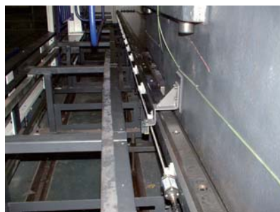
10mm dia. housing pipe mounting Order code: 1900951002 (Install for every 500mm)
